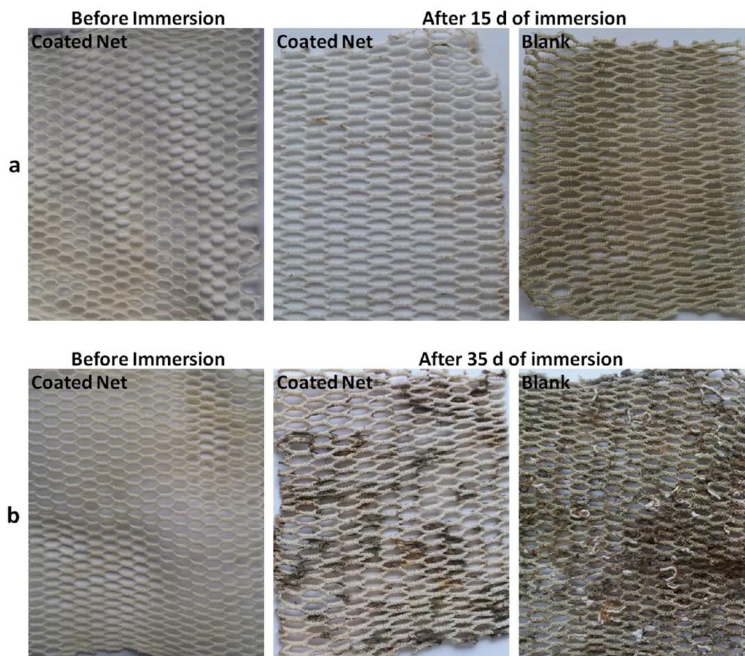
**Figure 8.** Photographs of the coated and uncoated nets (blank) after immersion in the sea environment for 15 and 35 days.
