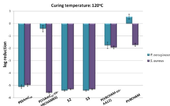
**Figure 7.** Antimicrobial effect of the membranes S2 and S3 after cross-linking at 120 °C, the copolymers P(SSAmC<sub>16</sub>-co-VBCHAM65) and P(VBCHAM-co-AA12), and the homopolymers PSSAmC<sub>16</sub> and PVBCHAM. The experiments were conducted after 24 h of contact with *S. aureus* and *P. aeruginosa* at 22 °C. Each bar represents the log reduction from three independent experiments done in duplicates (mean ± standard deviation).
