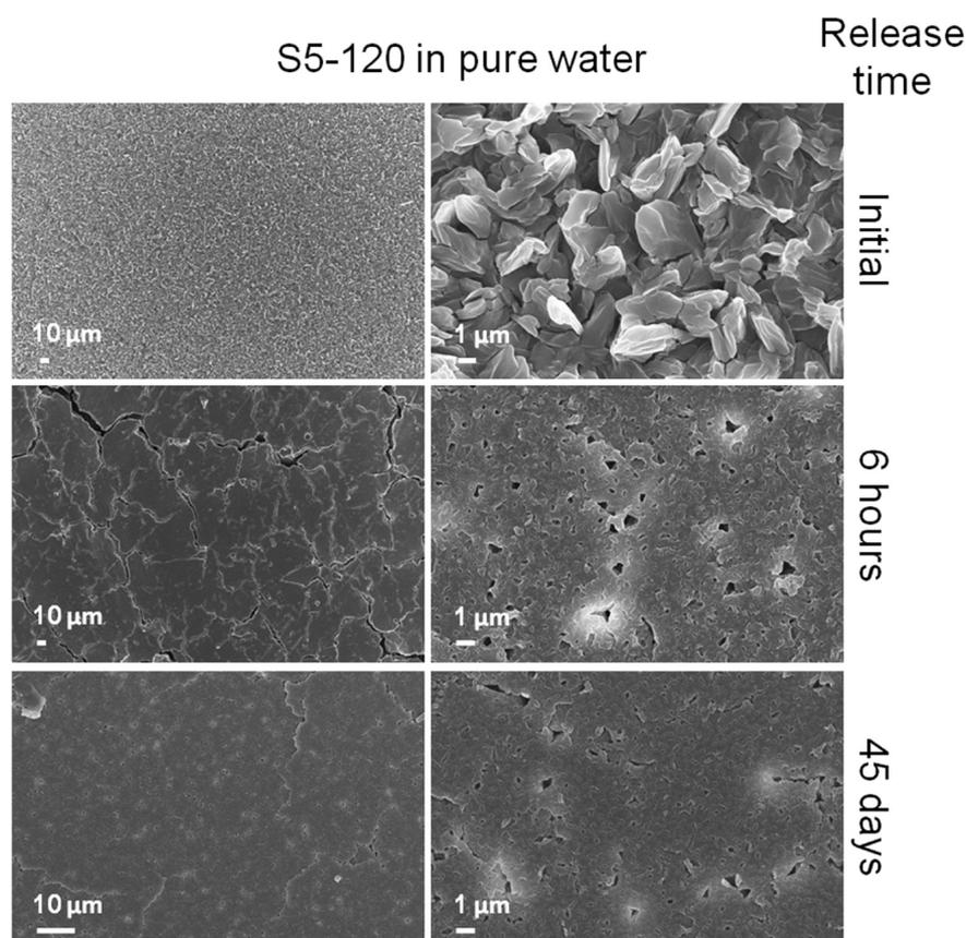
**Figure 6.** SEM of membrane S5-120 before and after immersion in pure water for 6 h and 45 days.
