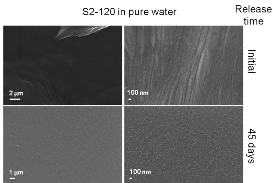
**Figure 5.** SEM of membrane S2-120 before and after immersion in water for 45 days.
