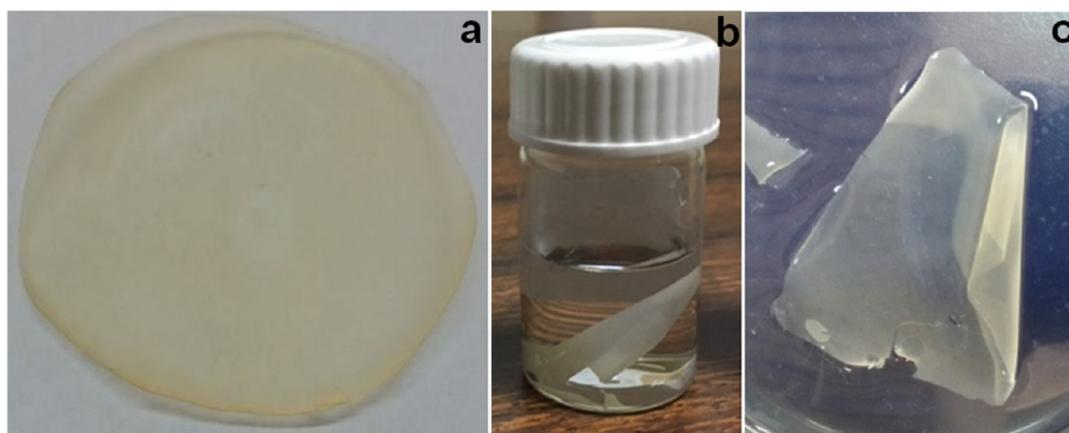
**Figure 3.** Appearance of (a) the membrane S5-120 after curing, (b) a piece of the membrane immersed in pure water for 30 days, and (c) a dried piece of the membrane after the release study.
