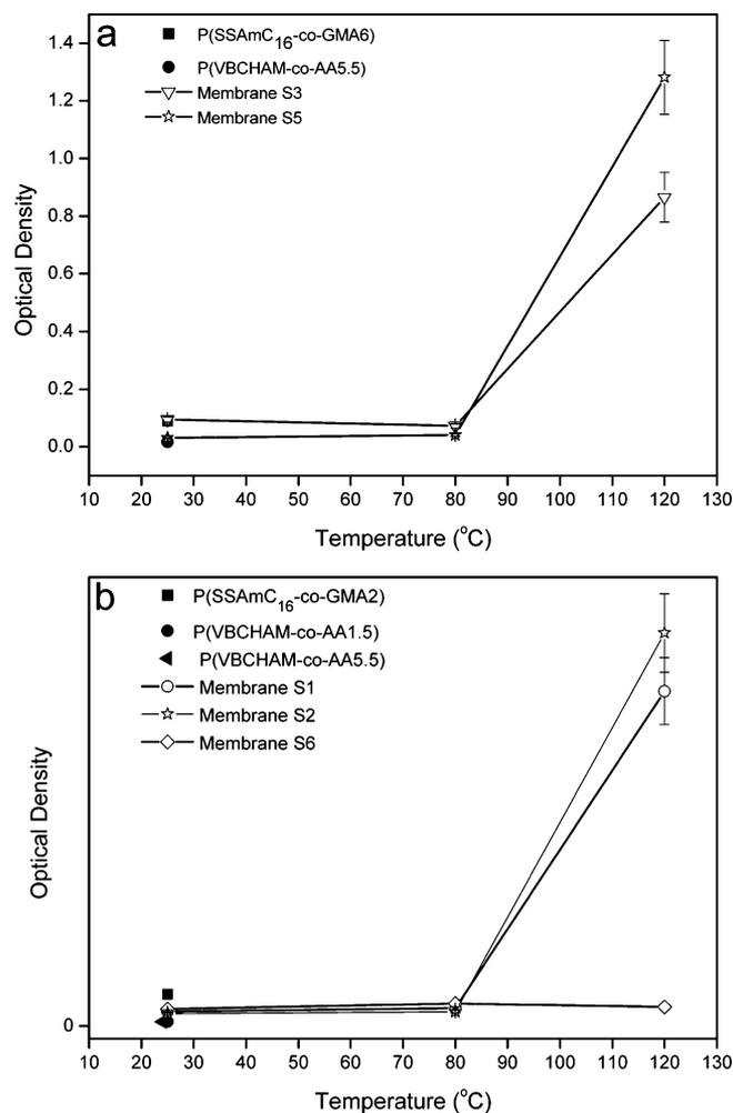
**Figure 2.** Turbidity studies of the membranes (a) S3 and S5, (b) S1, S2, and S6 versus curing temperature. The turbidity of solutions of the respective complementary copolymers is also shown. The copolymers/membranes were dissolved/dispersed in CHCl<sub>3</sub> at 1% (w/v) concentration.
