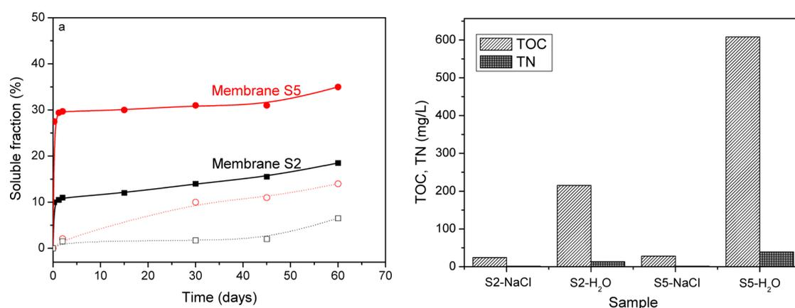
**Figure 4.** (a) Evolution of the soluble fraction of membranes S2-120 and S5-120 immersed in pure water (solid curves) and in an aqueous 1 M NaCl solution (dashed curves). (b) TOC and TN results of the aqueous media used for the release study of the two membranes for 60 days.
