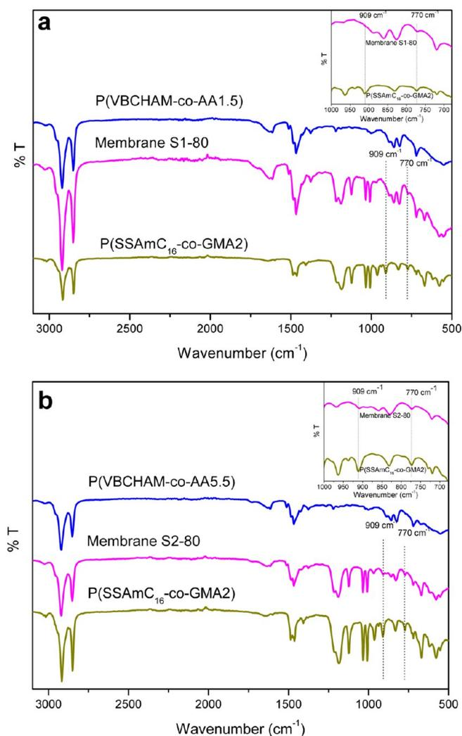
**Figure 1.** ATR-FTIR spectra of the membranes (a) S1-80 consisting of P(SSAmC<sub>16</sub>-co-GMA2) and P(VBCHAM-co-AA1.5) with a composition 15/85% (w/w) and (b) S2-80, consisting of P(SSAmC<sub>16</sub>-co-GMA2) and P(VBCHAM-co-AA5.5) with a composition 40/60% (w/w).
