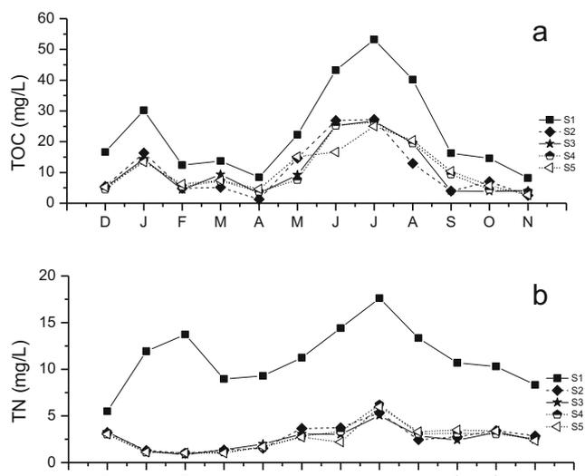
**Fig. 4** Monthly values of: **a** total organic carbon (TOC) and **b** total nitrogen (TN) in monitoring stations S1-S5
