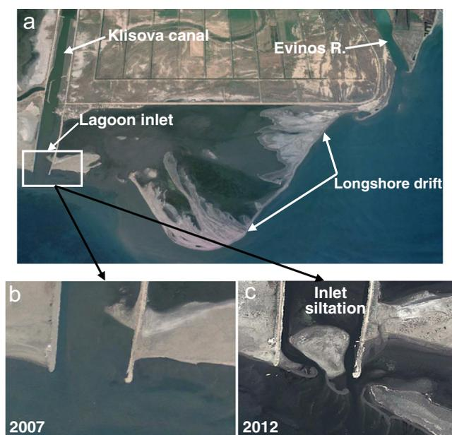
**Fig. 8** Aerial photographs showing: **a** the Klisova canal, the lagoon inlet and the Evinos R. delta, **b** the lagoon inlet in 2008 and **c** the lagoon inlet in 2012 with the sediments siltation as the result of longshore drifting
