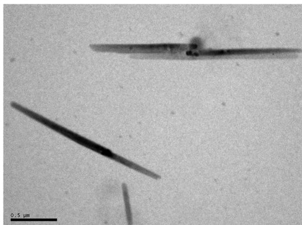
Fig. 7 TEM image of the diblock copolymer PtBA-*b*-PVBCHAM55.
