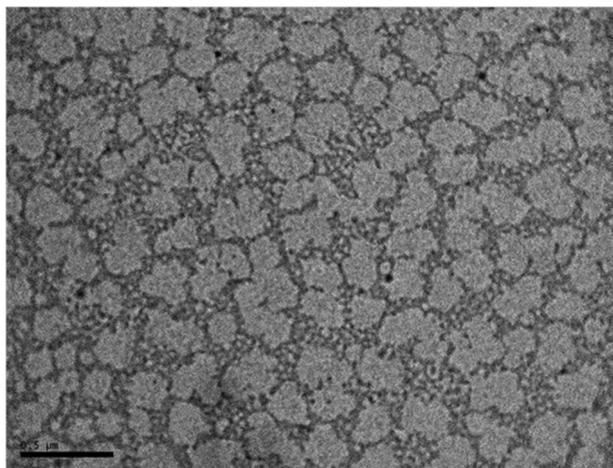
Fig. 8 TEM image of the diblock copolymer PVBCHAM10-*b*-PSSAmC<sub>16</sub>.
